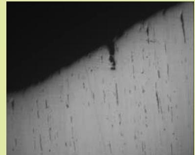
**Magnification:** 100X**Etchant:** - As polished condition**MOC:** SS 304**Component:** Gear box anchor bolt
