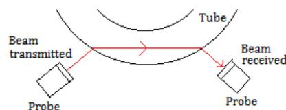
Figure 1 Principle of Attenuation Measurement, Ultrasound Inspection
