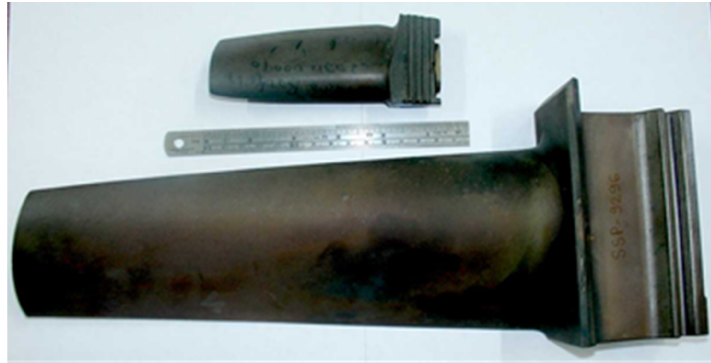
1st stage turbine rotor blades of an aero engine (top) and IGT (bottom).
