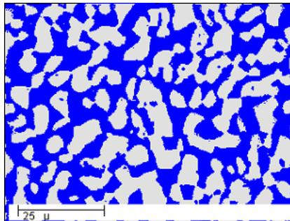
*Polarized image of austenite phase in duplex steel*
