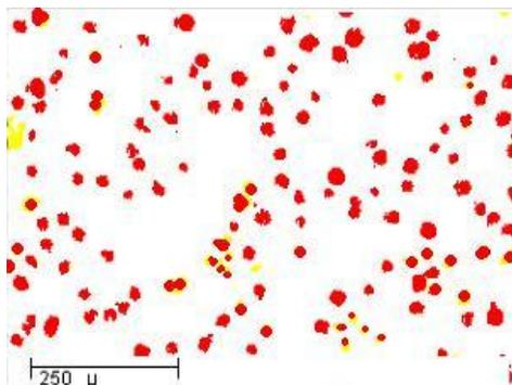
*Identification of Nodules in casting sample in As-polished condition.*
