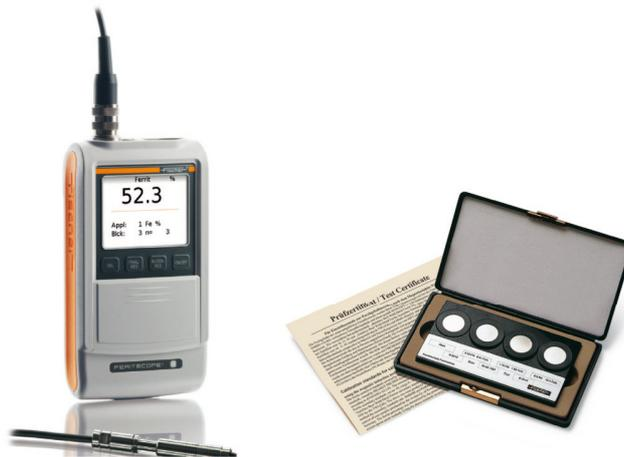
The FERITSCOPE FMP30 measures the ferrite content in austenitic and duplex steel according to the magnetic induction method. It is suited for measurements according to the Basler-Standard and according to DIN EN ISO 17655. Areas of application are onsite measurements, e. g. of austenitic plating as well as weld seams in stainless steel pipes, containers, boilers or other products made of austenitic or duplex steel.
