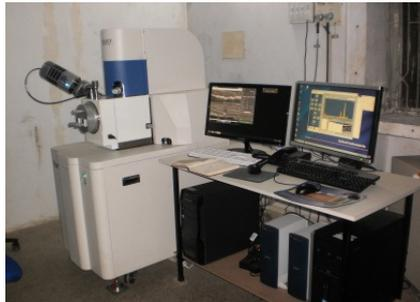
Using magnetic lens a focused Beam of electron is used to scan the small area of sample gives many benefits for imaging.
